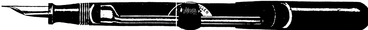
Sectional View showing Crescent Filler released, and the Elastic Ink Reservoir compressed ready for filling.
